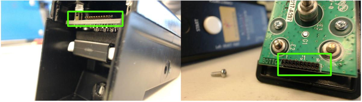
3. Once the pieces are lined up, take the screw you removed in step 2 and use it to screw the new front end to the base piece.
