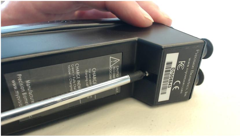
4. Perform a test with your static scanner. If the readings come out like in the exam below, remove the new front end and re-attach it, the pins can take a few tries to properly line up inside the device.
