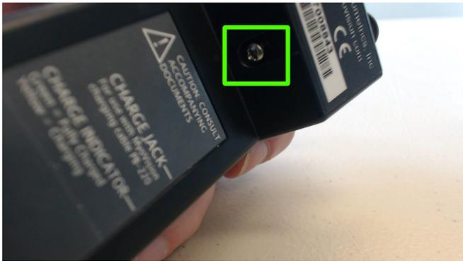
Unscrew it from the device and pull the front end piece off. You may need to give a gently wiggle to loosen. Make sure to keep the screw as you will need it to screw the new front end back to the base piece.
