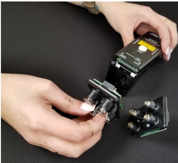
2. When placing the new front-end into place, make sure the tabs on the front end and slot for the tabs (highlighted in green in the images below) on the base piece are lined up. Make sure the front end is fully secure in the device.
